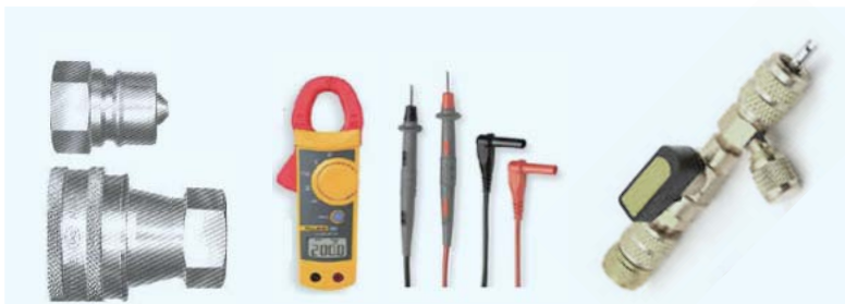
Figure 4.9 : Male and female quick coupler, Digital Clamp Meter and Core Removal Tool
