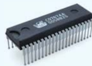
Figure 2.23: Integrated Circuit (microchips)
