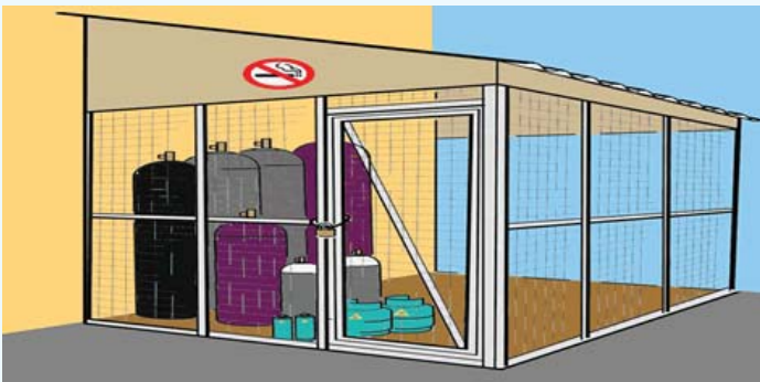
Figure 7.19 : Safety storage for flammable refrigerants
